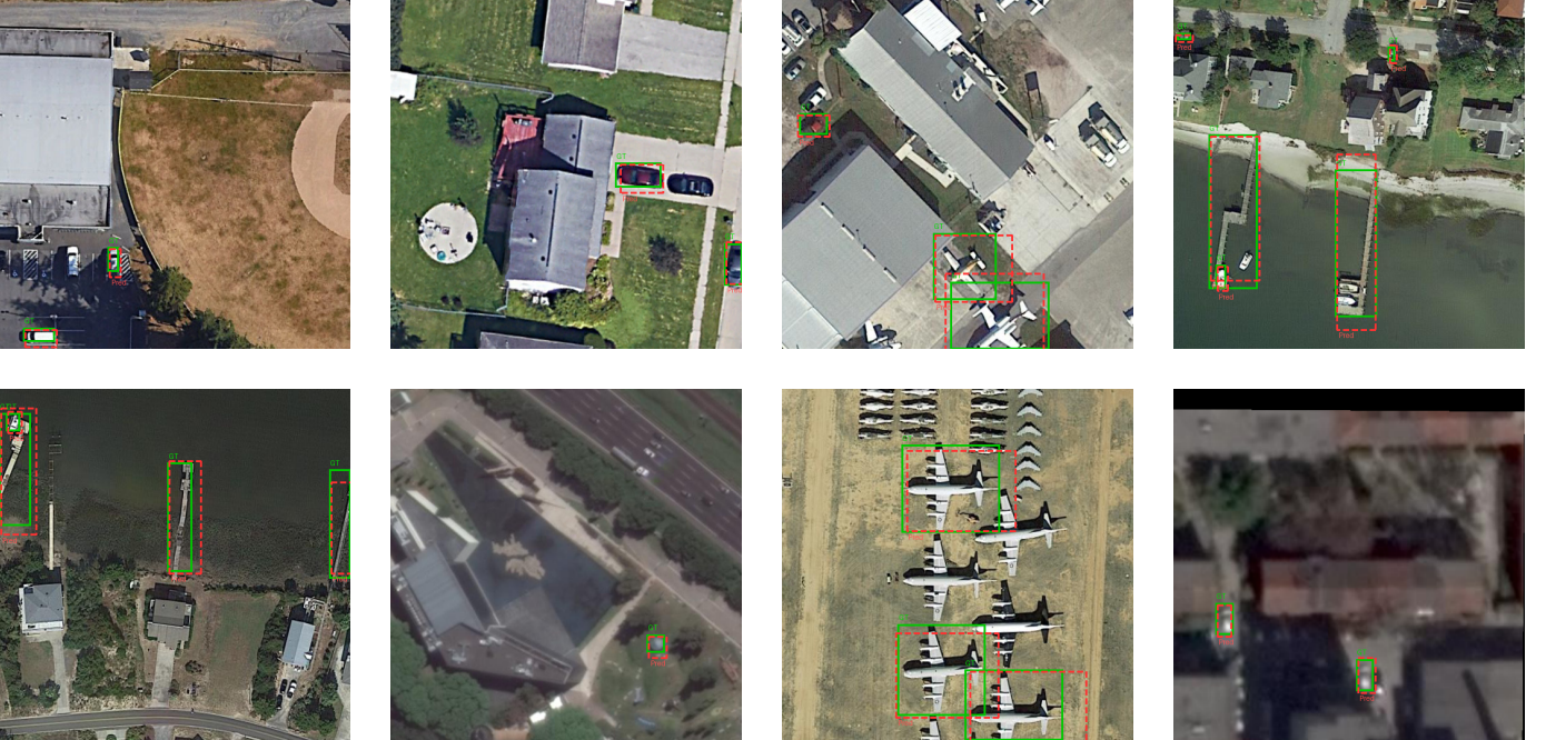
Fig. 6. Bounding box visualization results. Green solid boxes denote ground truth (GT), and red dashed boxes denote predicted boxes (Pred).
